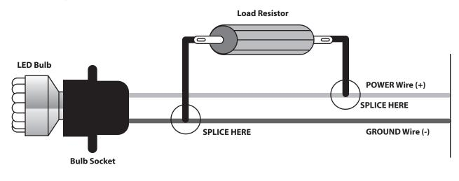
**If you have more than 2 wires** coming out of the bulb socket, you will need to isolate the **TURN SIGNAL** wires for the load resistor to work properly. Use a voltage meter or refer to a diagnostic manual to determine which **2 wires** (always 2, power and ground) carry the voltage for the turn signals. See diagram below.
