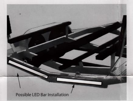
Step 3: Use the included tie straps to secure the wiring up underneath your trailer, working your way back up to the 4 pin trailer connector. Work your way to the front of the trailer near the hitch, keeping the wiring secured in order to avoid possible snags while towing. Be careful to avoid pinch points and moving parts. (if your vehicle does not have a 4 pin trailer connector, see Alternate Instructions)
