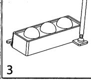
**Drill Pilot Holes** Insert Screws
