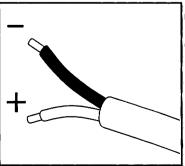
**Cut Off Plug To Connect To** 12 Volt Power
